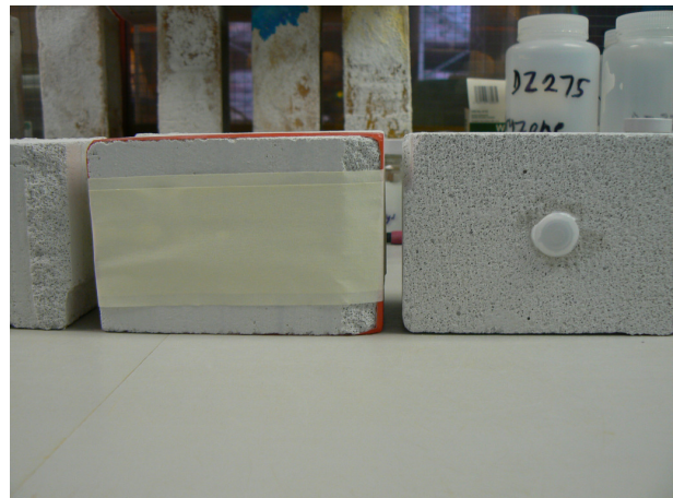
Photo 2: Tape is placed over the slot and the hole capped
